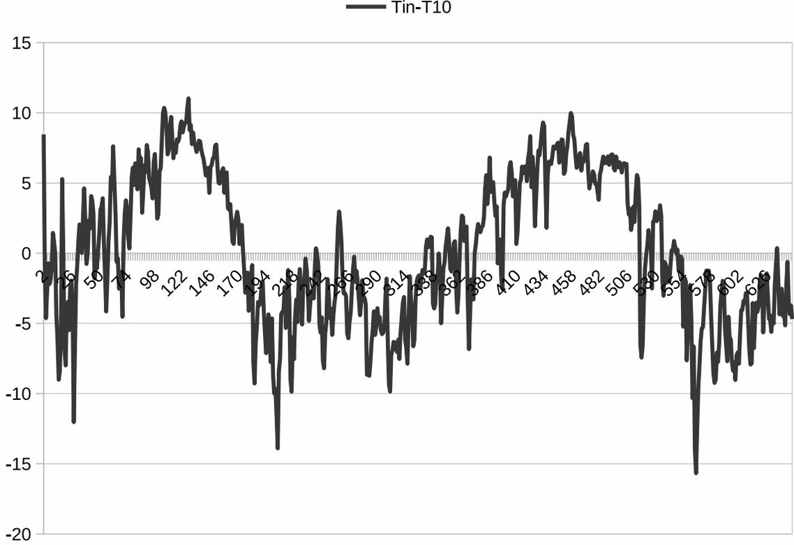
Figure 4: Difference between indoor air temperature  $T_{in}$  and temperature of earth 27" below top of slab  $T_{10}$
