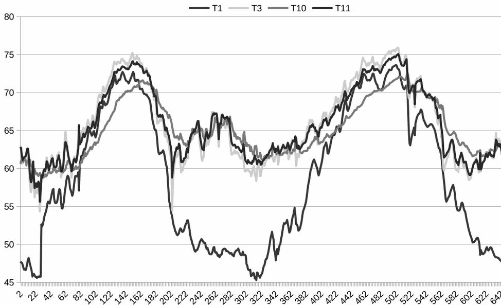
Figure 3: T1 edge of building 30" down, T3 in slab saw cut, T11 bottom of slab, T10 is 27" down, center of building.
