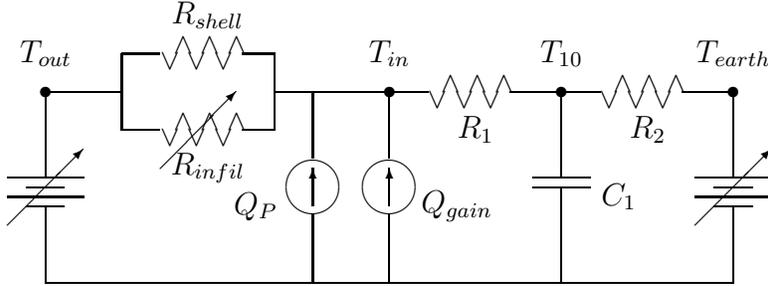
Figure 2: Simplified electrical model of heat flow in Morton building.
